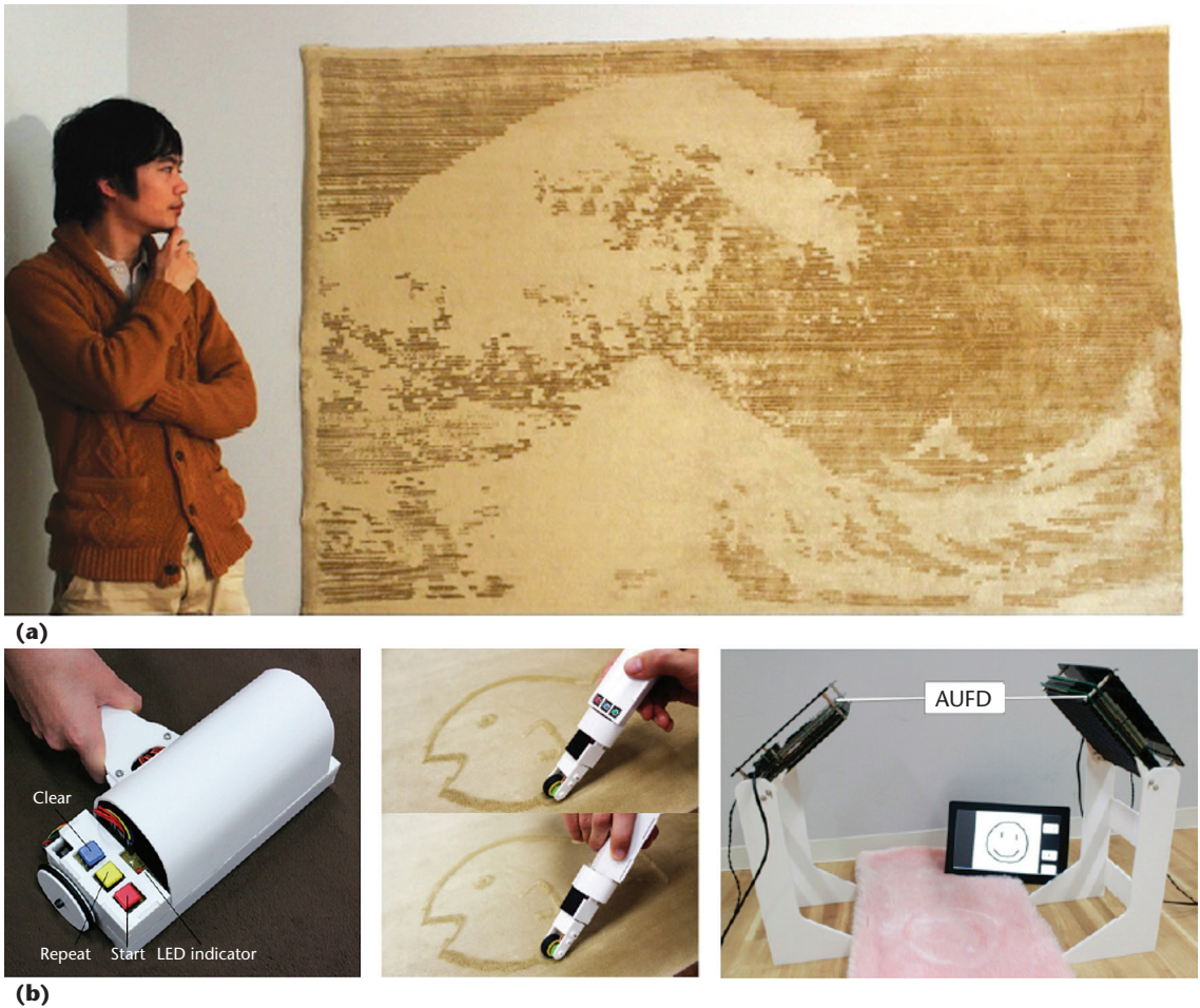
Figure 9. Graffiti Fur, devices for drawing on a carpet. (a) This technology can convert ordinary objects into rewritable computational displays using (b) a roller, pen, or pressure projection devices.
