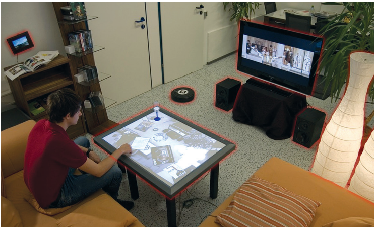
Figure 3. CRISTAL, a remote control system using augmented reality. Users can control various consumer electronics remotely using the touchscreen or graphical widgets, such as a slider.
